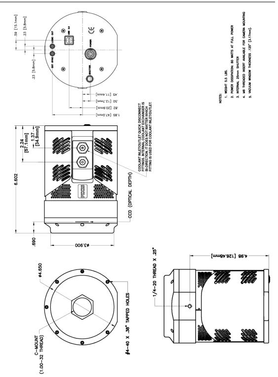
Figure 61. Fixed C-Mount: Internal Shutter (Liquid-cooled)
